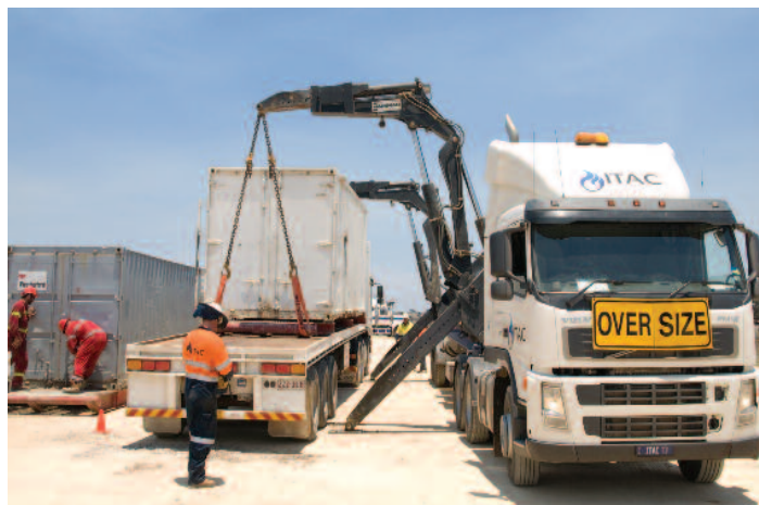
Lifting container from flatbed. Note the reach beyond the stabilisers.
