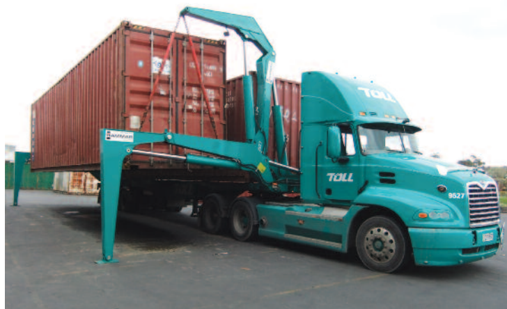
The 155HS stabiliser has a wide and high tunnel much like an “h” as noted in both photos on this page.
