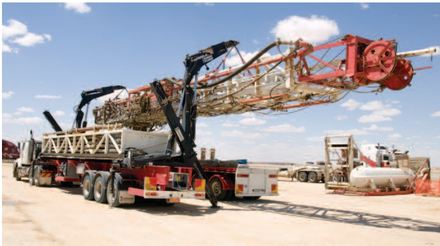
Hammar hard at work—a 23 m, 23 tonne drill rig mast being transferred to another trailer.
