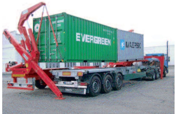
Double stacking is easy with the Hammar 155 Mega transfer
