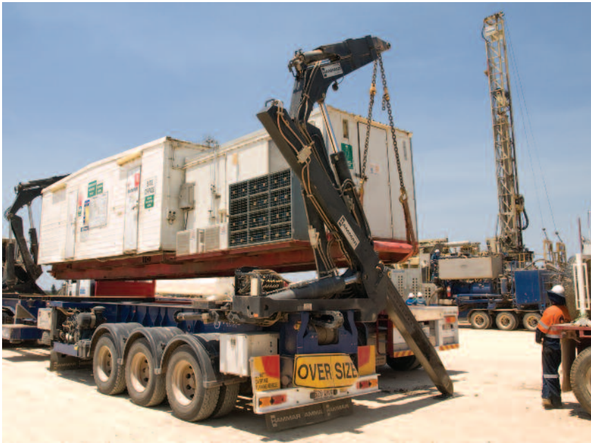
Site office loaded using the Hammar 151 C
