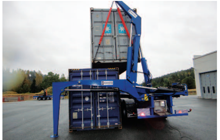
Double stacking is easy with the Hammar 155 Mega transfer
