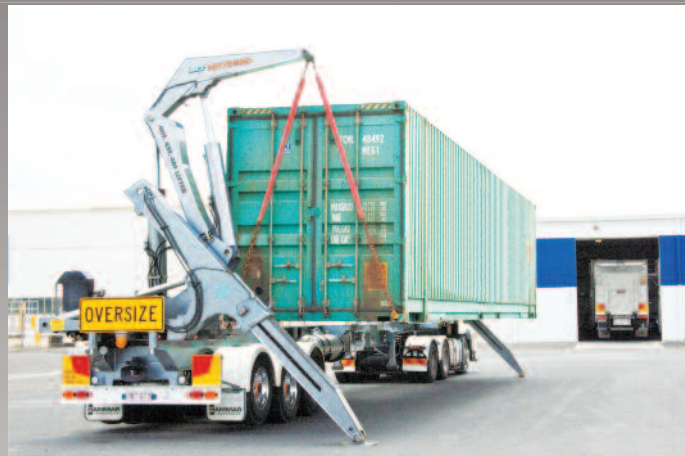
Handling a 48' container
