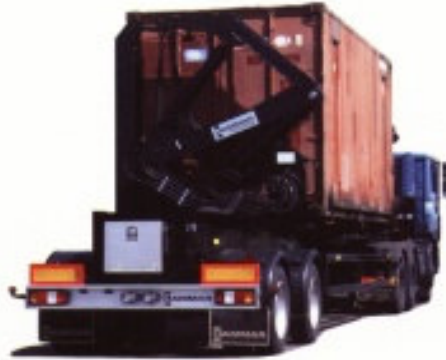
Hammar 160 S. The cranes are slid hydraulically on the semi-trailer frame, 20' - 40'. (S stands for sliding).
