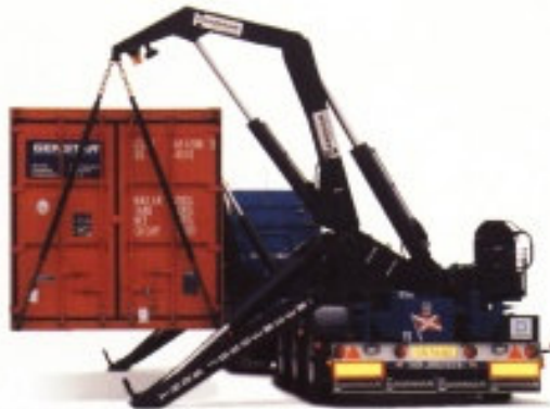
Hammar 160 HS can high stack any container on top of an 8'6" (2591 mm) high container. Shown here is a 20' - 45' adjustable version.
