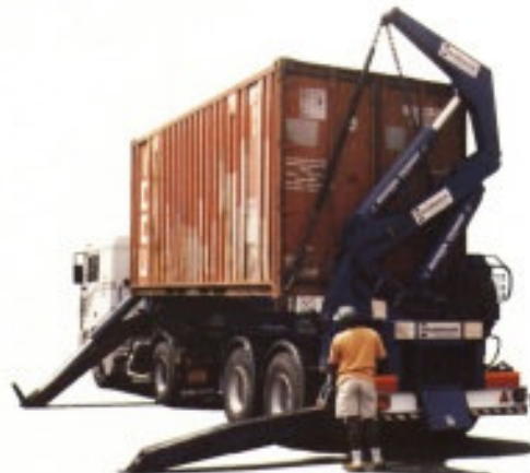
Hammar 167 HT is a high stacking model mounted on a telescopic trailer. (T stands for trombone). The rear stabilizer, placed low under the semi-trailer frame, makes transferring to or from railway cars and semi-trailers easy.
