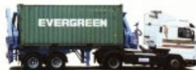
Hammar 151 HT. Here contracted to 20'. Suitable for transportation in confined areas with little space.
