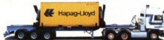
Hammar 151 HS with a 20' container. Adjusting the cranes between 20' and 40' takes only twenty seconds. All models are provided with remote controlled hydraulically adjustable cranes. As an option we can supply 10' - 48' capacity.
