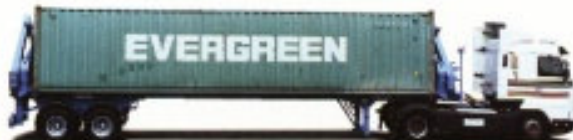
Hammar 151 HT. The length of the trailer frame can be adjusted between 20' and 40'. (T stands for Trombone).
