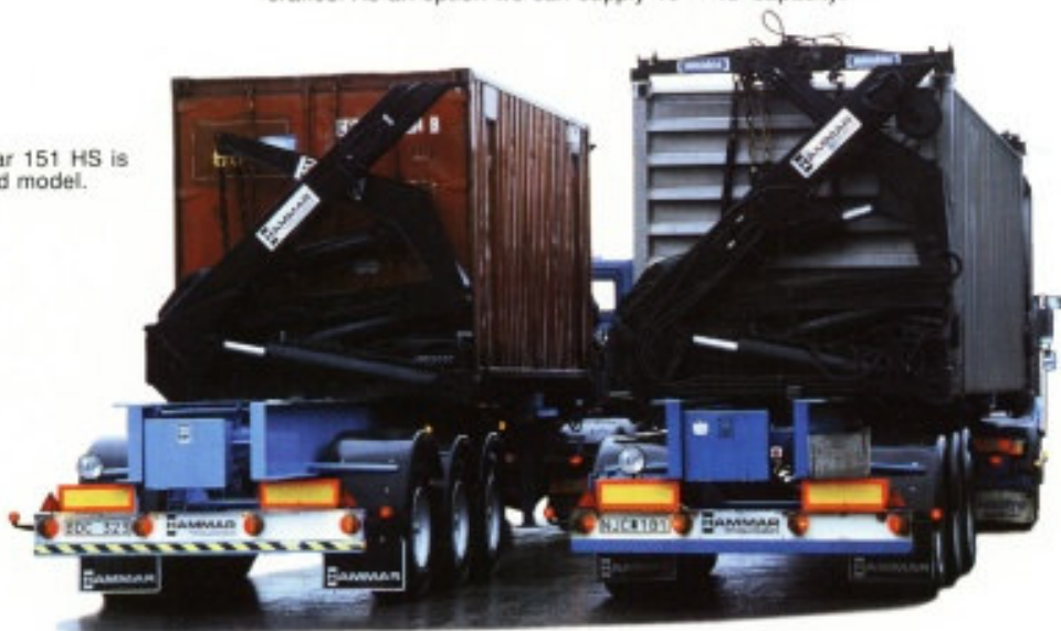
Hammar 151 HS with a 20' container. Adjusting the cranes between 20' and 40' takes only twenty seconds. All models are provided with remote controlled hydraulically adjustable cranes. As an option we can supply 10' - 48' capacity.
