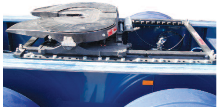
The chassis is fitted with an air-operated sliding turntable to cater for different B-Trailers
