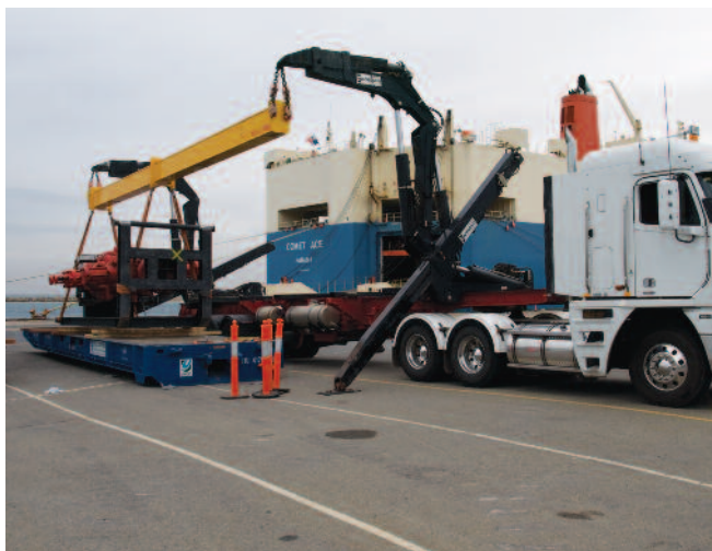
Loading from a mafi flat, just off-loaded from roro vessel (at the back)
