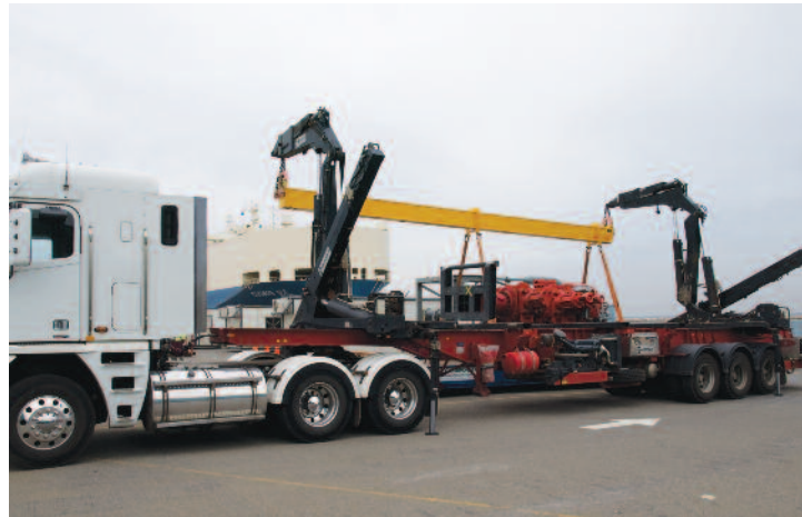
Plant without lifting points like this BOP can be loaded, using a lifting beam
