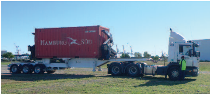
The Hammar A-Double system gives the added benefit of the ability to position 20’ containers to optimise weight distribution.
