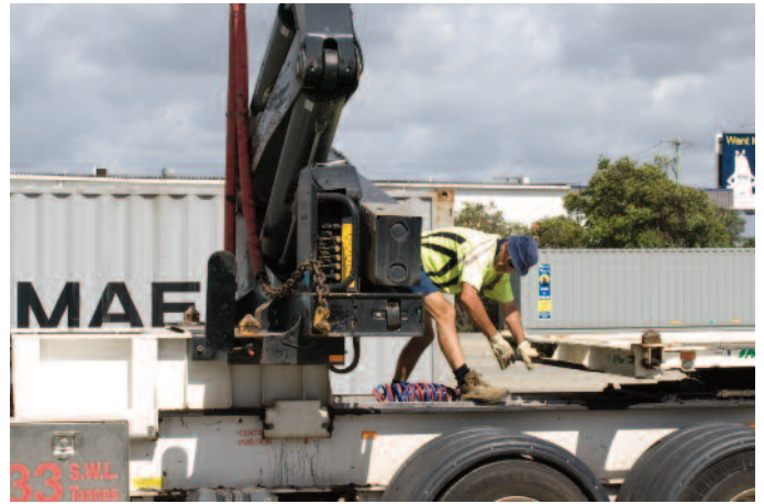
It is easy to connect and disconnect the B-trailer. This allows the driver to load two trailers in combination in just 20 minutes.
