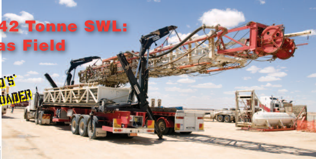
A 23 m, 23 tonne drill rig mast being moved to another trailer
